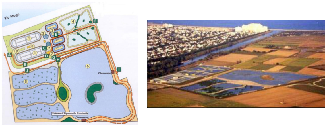
Figure 11-3. Scheme and aerial view of the Empuriabrava WWTP, the lagooning system and the constructed wetlands (WWRRS). Source: Seguí, L., et al., 2007.
